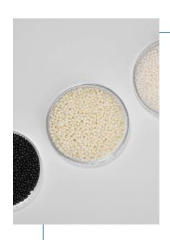
TPV are mainly consisted of different species of EPDM/PP with set composition ratios and vulcanized (or dynamically crosslinked) to afford the elastomers in a wide range of hardness and with unique properties.
