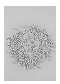
TPU is a copolymer made from polyol and MDI. It is biodegradable in natural environments, making it an eco-friendly material. TPU can replace plastic products.
